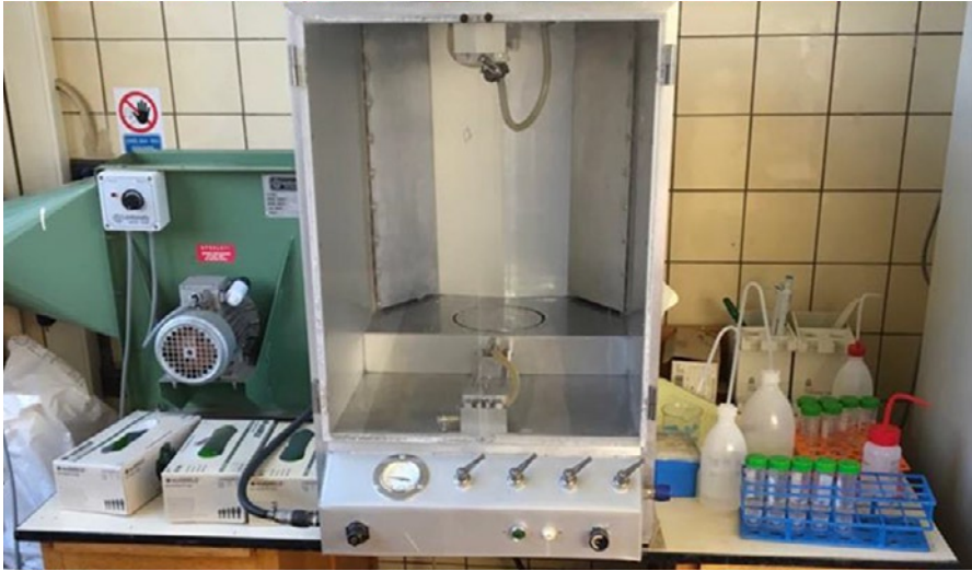
Figure 1. Cornelis spray tower, at Ghent University's Laboratory of Agrozoology (Ghent, Belgium).
