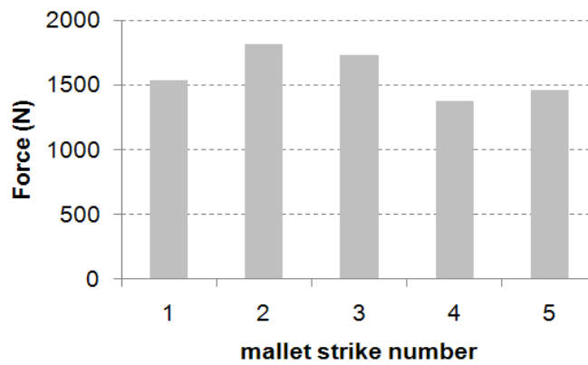
Figure 9: Maximum Impaction Forces of the Strikes for the D-2 Implantation.
