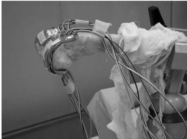
Figure 3: Photograph of the D-1 Bone Clamped Horizontally, with Strain Gauged Femoral Component Implanted.
