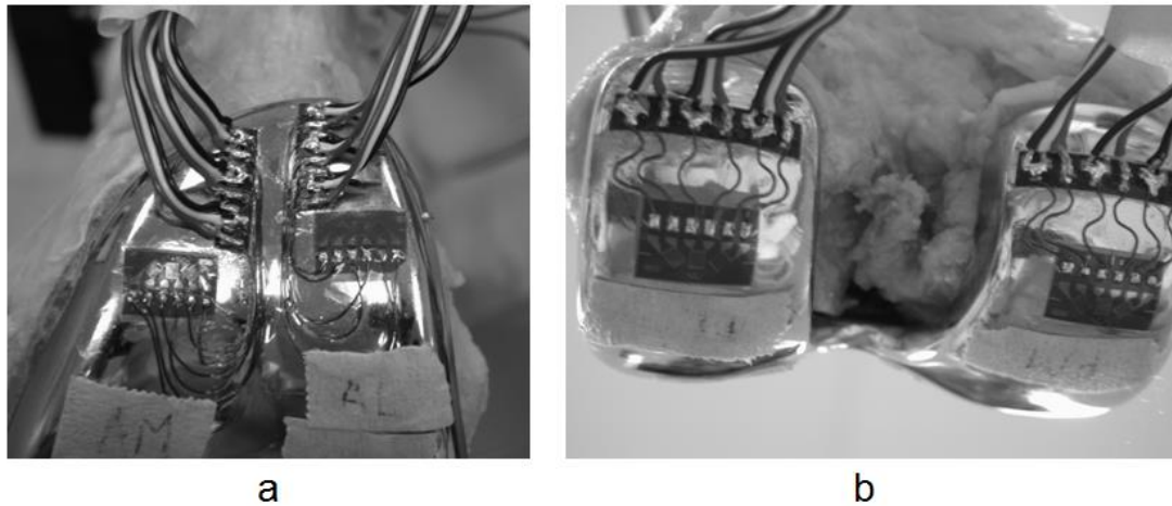
Figure 2 Photographs of Strain Rosette Locations. a) Anterior view showing rosettes on anterior shield, b) Posterior view showing rosettes on each posterior condyle.
