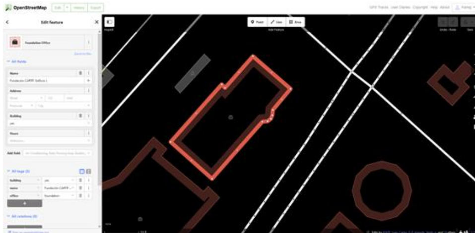
Figure 1 Example of building with three tags defined (down left), including building, name and type of office
