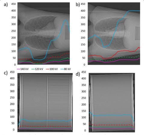
**Fig. 2** Axial mAs profiles for scans at each kV for **a** Lungman, **b** Lungman plus fat, **c** Esser and **d** NEMA IQ phantoms. Optimal kV determined by 'CARE kV on' mode shown with dashed profile. Minimum deliverable 13 mAs effective using selected protocol
