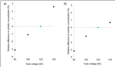
Fig. 4 Differences in a maximum and b mean activity concentration for each kV relative to 120 kV reference in Lungman plus fat. Data points also corresponding to 'CARE kV on' shown with blue markers
