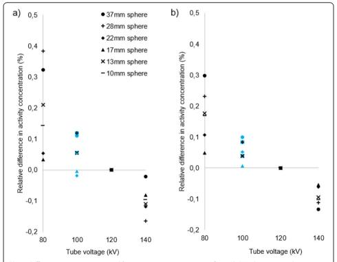
**Fig. 6** Differences in **a** maximum and **b** mean activity concentration for each kV relative to 120 kV reference in NEMA IQ phantom. Data points also corresponding to 'CARE kV on' shown with blue markers. There are 6 data points per kV setting corresponding to VOIs over the 6 spheres with some data points overlapping, particularly at 0.00% difference in measured activity concentration
