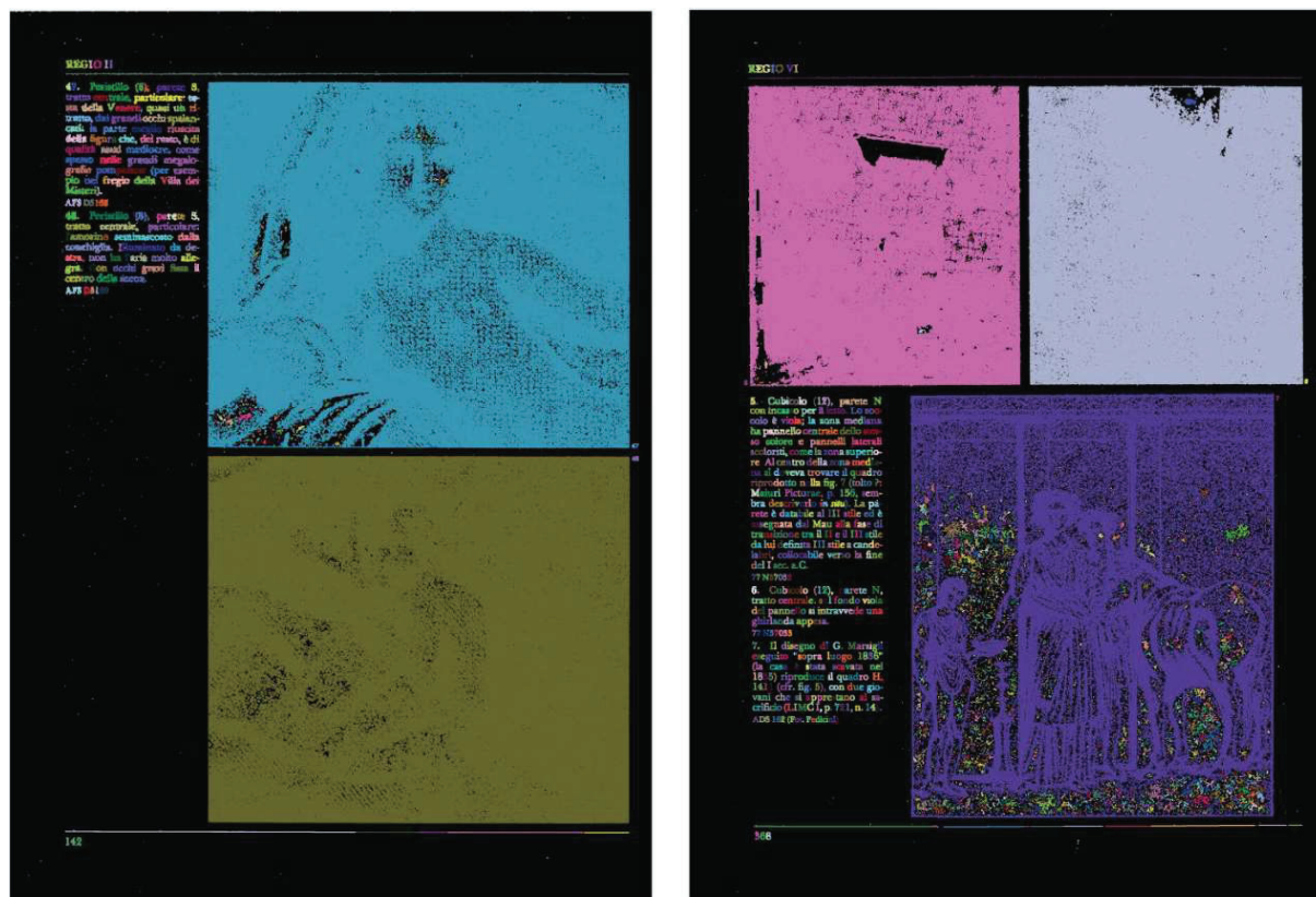
Figure 8: Connected Components Two examples of image of page scans after the average blur and connected component function applied. Each color corresponds of a different connected cluster.
