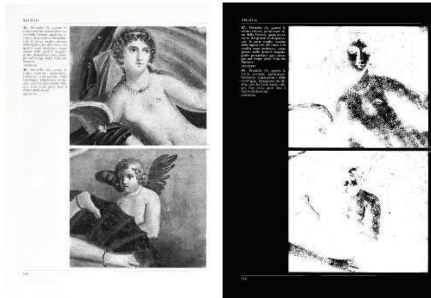
Figure 4: Threshold Binarization, Successful Example. Example of a binarization putting all the background pixel to 0 (any pixel with a higher value than 220) and the foreground to white. On the left side is the original page and the binarization result is on the right.
