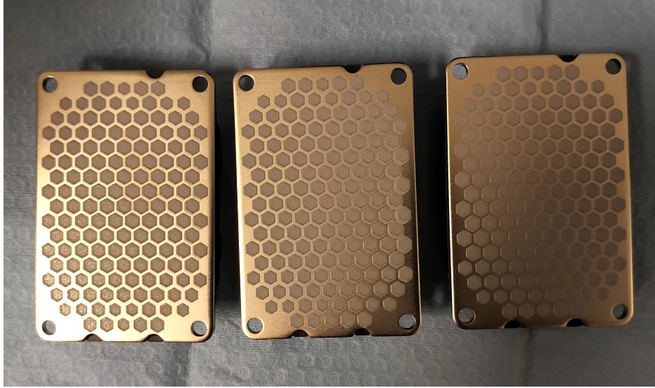
Figure 2.9: XM3 Base Plates with TIM Applied
