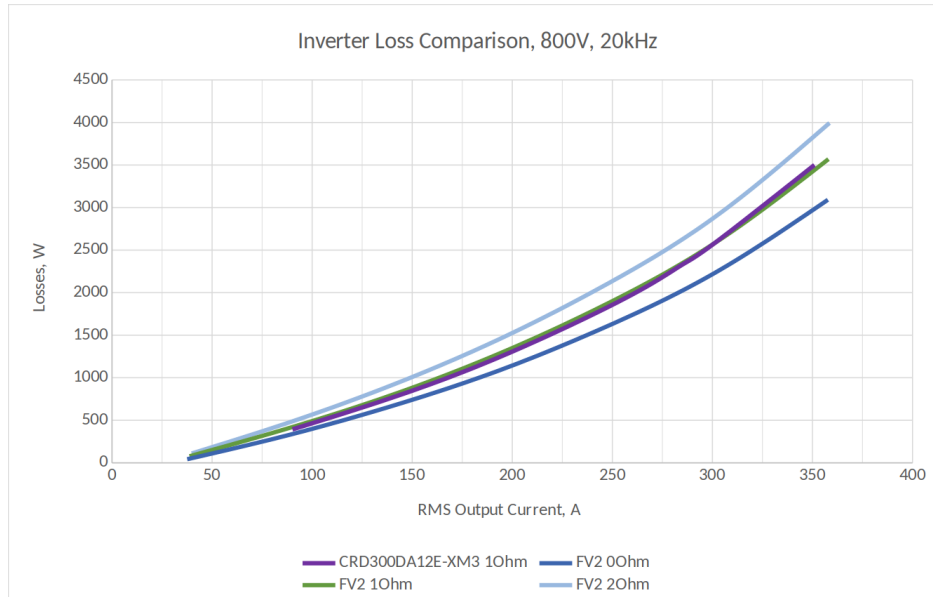
Figure 5.32: Comparison of losses at 800 V, 20 kHz with Various Gate Resistors
