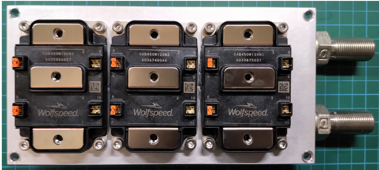
Figure 2.7: XM3 Power Modules Mounted on Cold Plate
