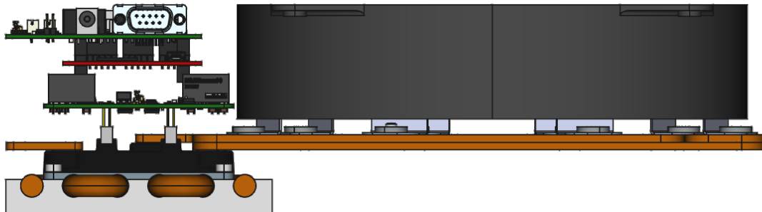
Figure 4.2: Design Option B with Capacitor Above Bussing
