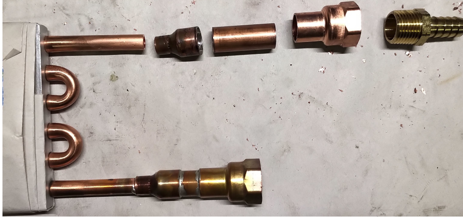
Figure 2.5: Cold Plate Pipe Adapters and Fittings Before and After Soldering
