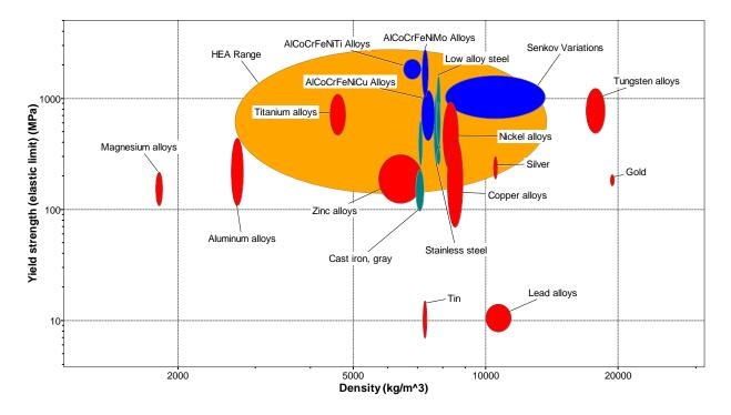
*Figure 3* – Ashby Diagram of Metal Alloys, with alloys of interest labeled, created on GRANTA EduPack 2020. [4][5]
