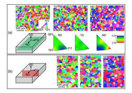
Figure 7 – Cross-sections of a cold rolled sample of the Senkov alloy, colored by orientation, and inverse pole figures to show orientation concentration [16]
