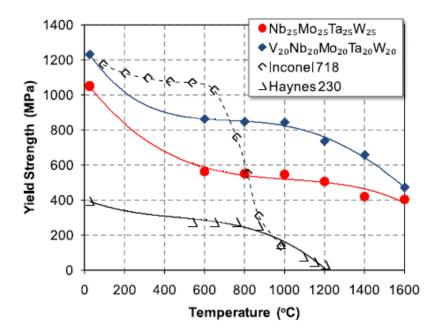
Figure 6 - Graph of strength retention of NbMoTaW and VNbMoTaW as temperature increases [21].
