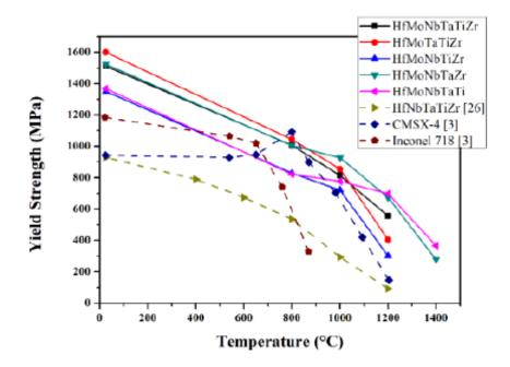
Figure 5 – Graph of the strength retention of HfMoNbTaTiZr alloys as temperature increases [20].
