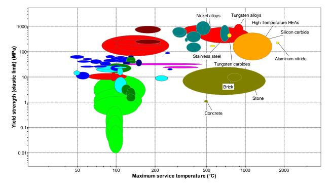
Figure 4 – Ashby Diagram Comparing Maximum Service Temperature with Yield Strength, overlayed by the corresponding scatterplot of High Entropy Alloys, created on GRANATA EduPack 2020 [4][5].
