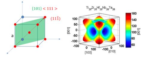
Figure 5 and 6 – A diagram showing the slip system of the Senkov alloy and an indicatrix of the Young's Modulus of the Senkov alloy depending on direction [15]
