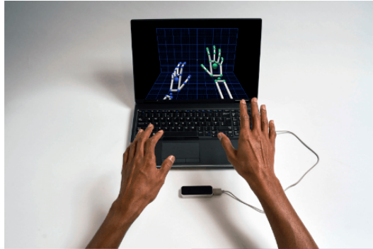
Figure 3. Ultraleap hand tracking with Leap Motion controller. Retrieved from " https://www.ultraleap.com/tracking/ " with permission.
