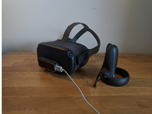
Figure 2. Ultraleap Leap Motion controller attached to Oculus Rift S with 3D printed mount.
