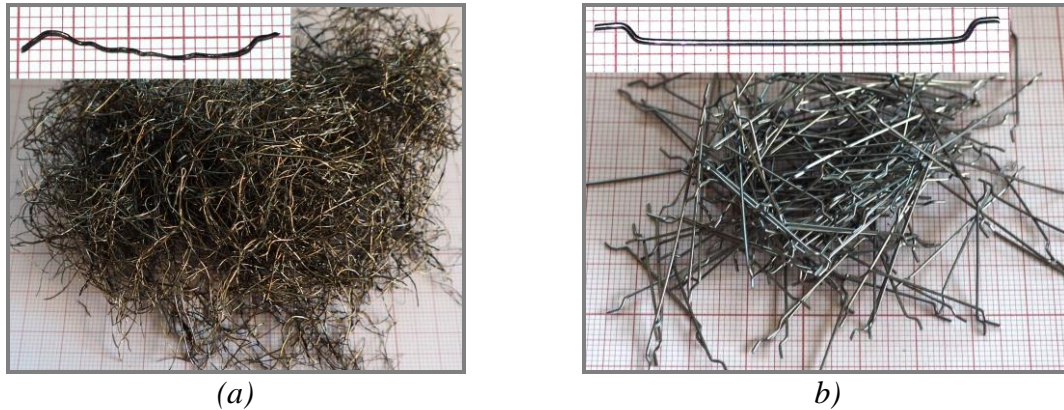
Figure 1 – General view of multi fibres and the geometry of a single fibre: (a) Recycled Steel Fibres: (b) Industrial Steel Fibres
