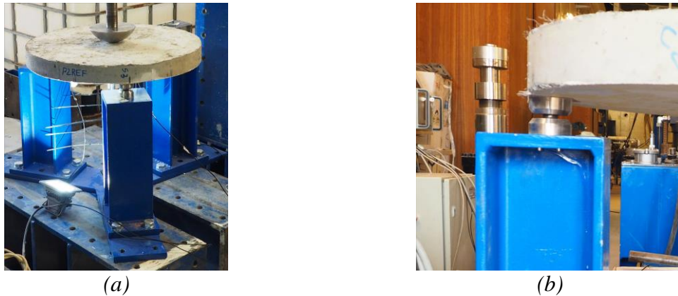
Figure 4 – Round panel test: (a) Test setup, (b) One of the three pivots of the supporting system for RPT
