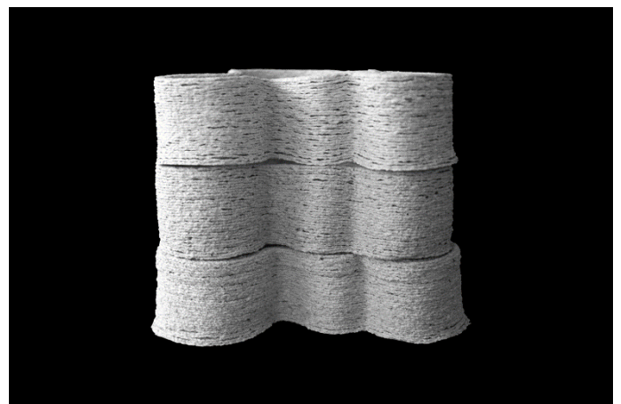
Figure 8. Final finishing of the AM Aalto pieces, printed with mixture B.1. Upper piece (15gr of sawdust), central piece (45gr of sawdust) and lower piece (30gr of sawdust).
