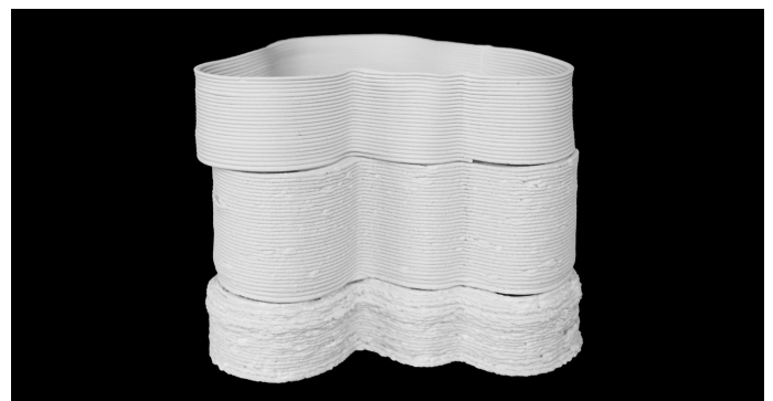
Figure 10. Top - ceramic paste, middle - ceramic paste and 25 gr of cellulose) and bottom - ceramic paste and 75 gr of cellulose.
