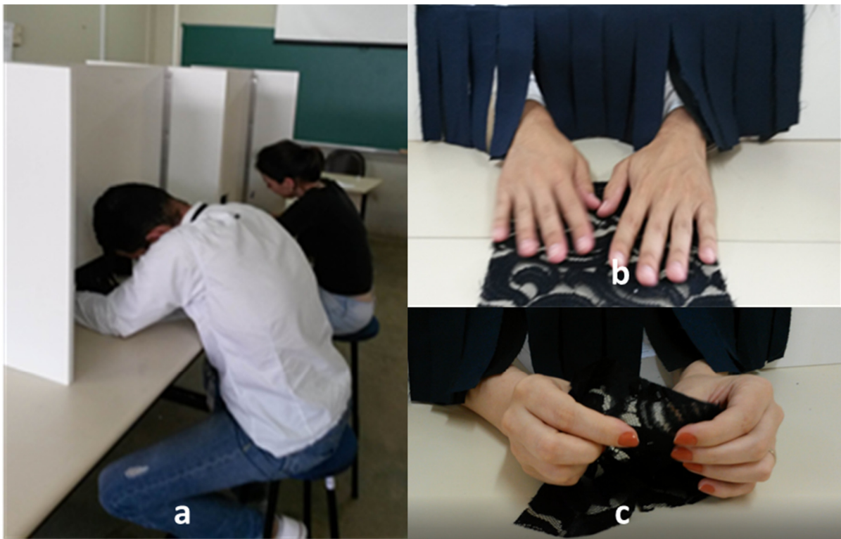
Figure 1. (a) Sensory evaluation cabin; (b) Touching one side of textile sample (c) Touching with both hands both sides
