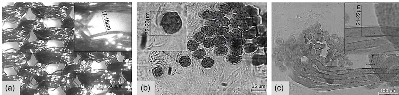
FIG. 7. Selected PLM images of: (a) J-A structure before laminate formation and measuring monofilament thickness (inset); Measuring the thickness of embedded monofilament in (b) P-R-15 laminate composite; (c) P-J-15 laminate composite.
