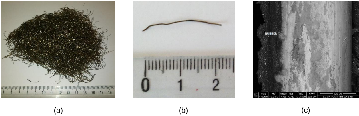
Figure 1 - Recycled steel fibers: (a) general view of multi fibers (b) general view of the geometry of a single RSF (c) SEM micrograph of the surface of a single RSF (Reference)
