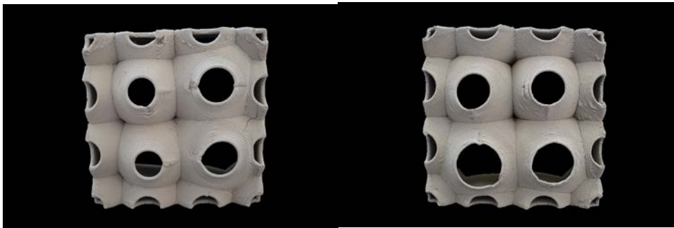
Figure 4: Same block produced with stoneware paste (left) and a mix of stoneware paste and cellulose (right).
