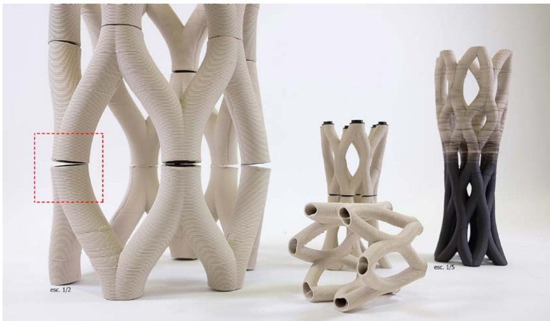
Figure 7: Ficus column system manufactured in ACLab at 1/5 and 1/2 scale
