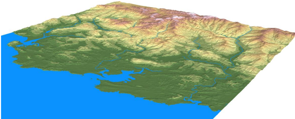
FIGURE 2: detail of the Digital Terrain Model (DTM) created from the Digital Elevation Model (DEM) generated for GIS analyses.
