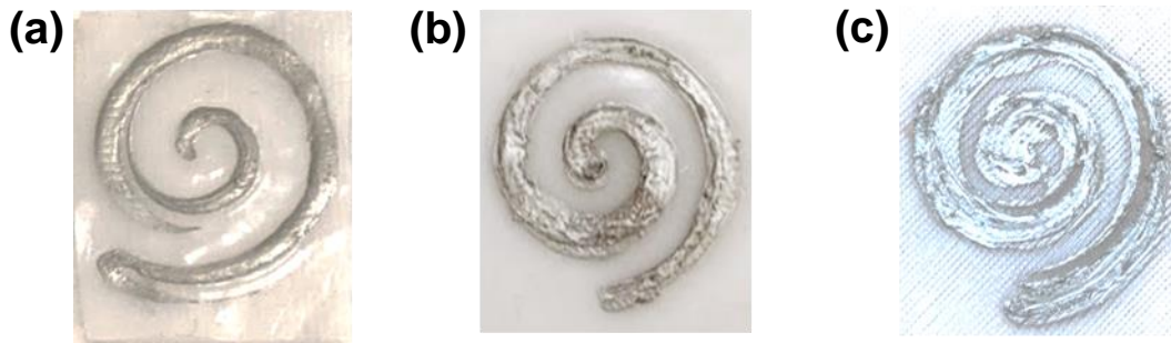
Figure 3.5: Prints of the single, double, and triple width inductors on PCL substrate.
