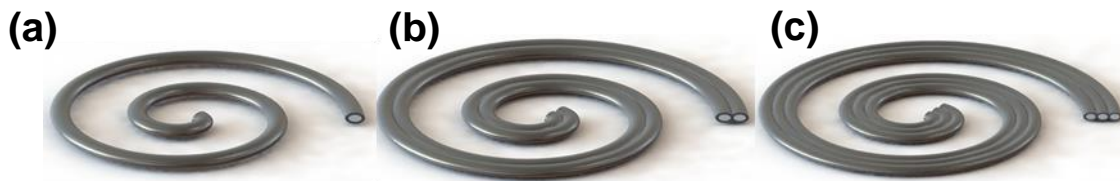
Figure 3.2: CAD renderings of the three designs. Thickness has been exaggerated to emphasize the core. Single, double and triple widths (a,b,c respectively) are shown.
