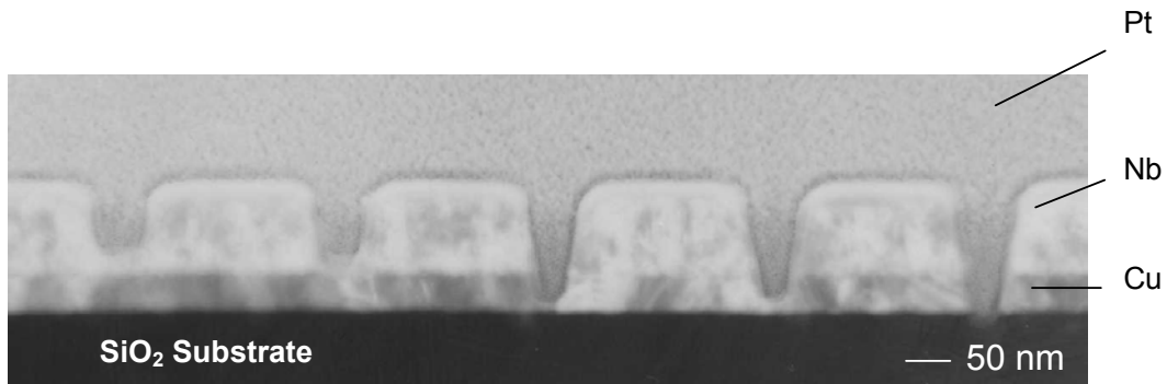
Figure 4.5: Bright field TEM image of (from left) 9, 10, 11, 12, 13 s cuts into a 125 nm Nb 50 nm Cu bilayer.
