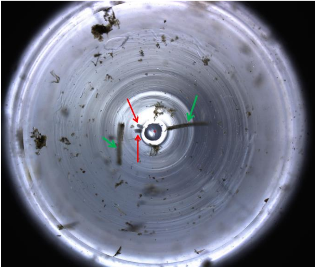
Figure 2-13 Representative image captured from the FECPAK G2 Micro-I of an equine faecal sample (Replicate 3 at 6 minutes accumulation). Image represents the central 3 mm of the well, which is the visible field of view. Red cross marks the centre of the image (added by Micro-I software), strongyle eggs marked by red arrows, examples of debris marked by green arrows.
