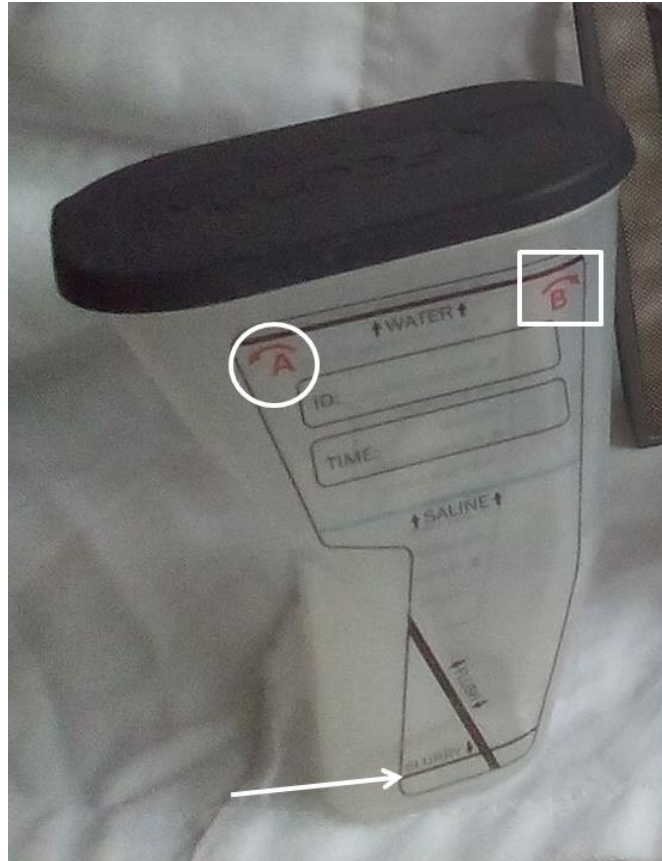
Figure 2-9 The FECPAK G2 Sedimentor (Techion Ltd, Dunedin NZ). The 12 ml faecal slurry line is highlighted with an arrow. Also highlighted is side A (circled) for discarding supernatant and side B (boxed) for pouring off the final sample preparation prior to imaging on the Micro-I or slide.
