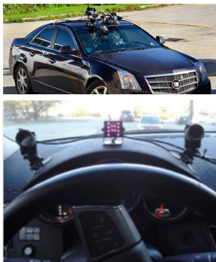
Figure 3.2: (top): Forward stereoscopic vision system on rooftop. (bottom): Infrared gaze tracker.
