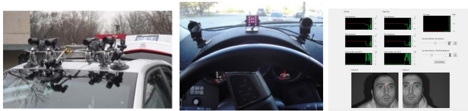
Figure 4.1: (left): Forward stereoscopic vision system on rooftop , (center): 3D infra-red gaze tracker , (right): The faceLAB system interface from SeeingMachines
