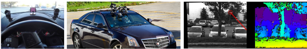
Figure 2.1: a) (left): 3D infrared gaze tracker ; b) (center): Forward stereoscopic vision system on rooftop ; c) (right): Driver PoG and LoG expressed in the reference frame of stereoscopic vision system and corresponding depth map.
