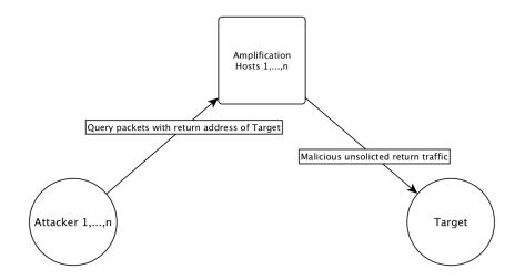
Figure 1.3. A DDoS amplification attack.
