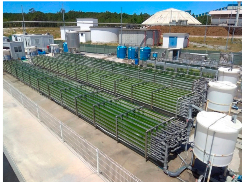
Figure 1. Pilot-scale tubular photobioreactors (PBRs) used in the trials with 2.6 \text{m}^3 of working volume (Allmicroalgae, Pataias, Portugal).
