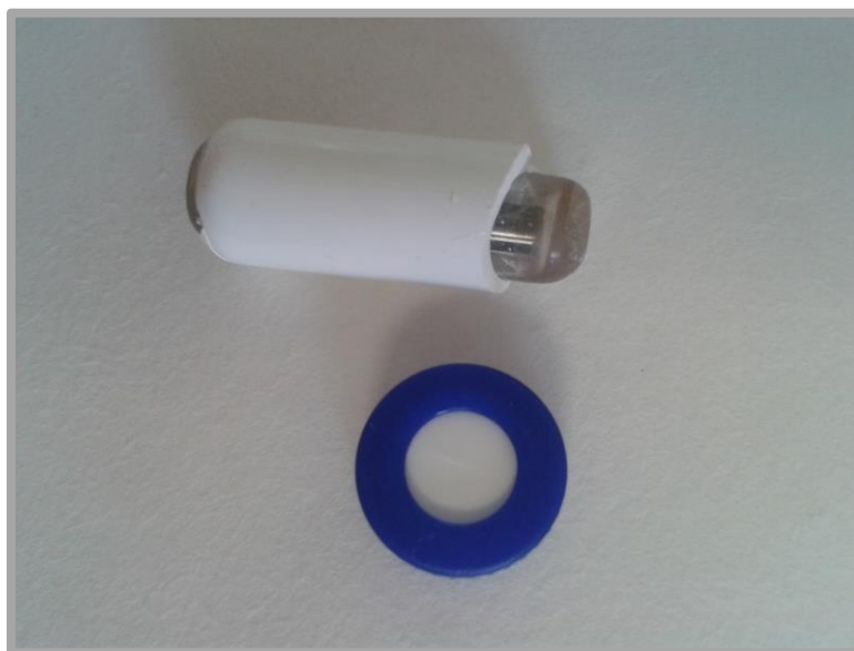
Figure 2: Magnetic molecularly imprinted stir bar (MMISB) developed for the extraction of patulin; the screw cap was placed below the stir-bar to illustrate its size.
