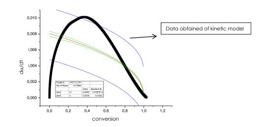
Figure 1. Reaction rate versus conversion
