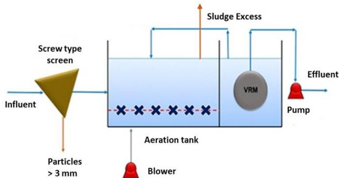
**Figure 7.1.** Flow diagram of the wastewater treatment plant with a membrane unit
