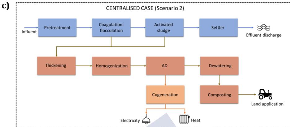
**Figure 8.1.** Centralised neighbourhood scheme: a) general configuration; b) system boundaries for Scenario 1 (WWTP of Santiago de Compostela); c) System boundaries for Scenario 2 (centralised case with AD unit)
