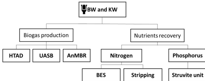
**Figure 1.4.** Main technologies for the treatment of BW and KW. Abbreviations: HTAD: high temperature anaerobic digestions; UASB: upflow anaerobic digestion; AnMBR: anaerobic membrane bioreactor; BES: bioelectrical systems
