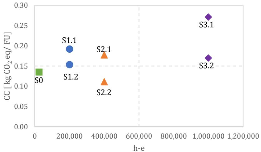
**Figure 2.3.** Comparison of the CC outcomes with and without biogas losses (FU: 1 ton of mixed sludge). Symbols: S0 (□): small plant; S1.1 and S2.1 (○): medium plant without biogas losses; S1.2 and S2.2 (△): medium plant with biogas; S3.1 (◇): large plant with biogas losses; S3.2 (◇): large plant without biogas losses.
