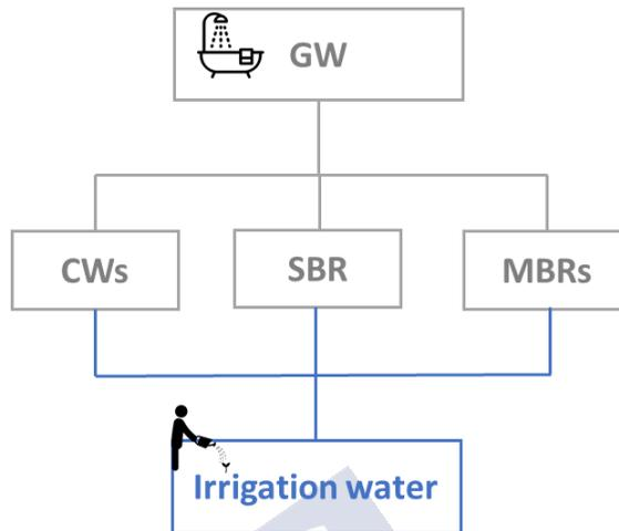
**Figure 1.3.** Most commonly used technologies for the treatment of greywater. Abbreviations: GW: grey water, CWs: constructed wetlands, SBR: sequencing batch reactors and MBR: membrane bioreactors.
