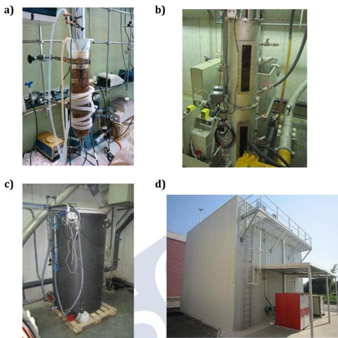
**Figure 6.2.** Different scales of the ELAN<sup>®</sup> process: a) Laboratory scale: 1.5L, b) Pilot Plant 1: 200L; c) Pilot Plant 2: 1.2m<sup>3</sup>; d) Full-scale: 115m<sup>3</sup>
