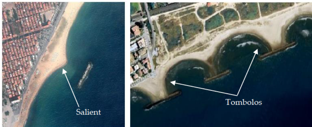
Figure 2.23 Example of a 'salient' (left) and a series of 'tombolos' (right) (Deltares- GFDRR, 2016)
