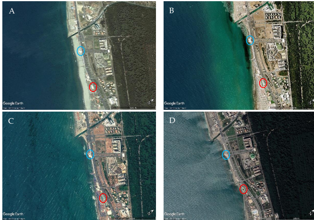
Figure 2.29 Armored river's mouth at Ostia (Central Tyrrhenian coast of Italy); (A) The Ostia's littoral in 2003; (B) Ostia's littoral in 2007; (C) Ostia's littoral in 2010; (D) Ostia's littoral in 2020. Images source: Google Earth.
