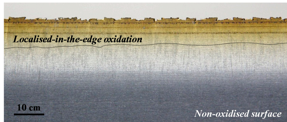
Figure 1. General view of the localised-in-the-edge oxidation of an AISI 430 ferritic stainless steel after bright annealing.
