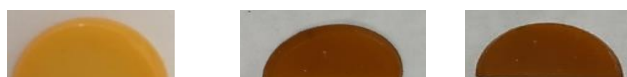
Figure 4.3.9 Sensor responses when exposed to a 20 ppmv ammonia atmosphere at 75 and 88 % humidity conditions compared to the reference blank sensor (left), which presented the same response between 51 and 88 % humidity conditions.
