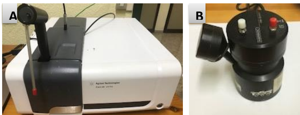
Figure 3.1 A) Cary 60 UV-Vis Spectrophotometer with B) Remote Diffuse Reflectance Accessory (DRA) accessory.
