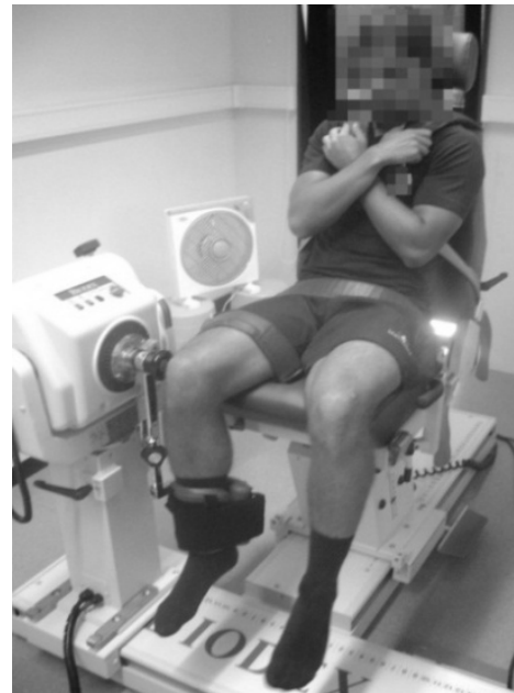
Figure 1. Positioning in isokinetic dynamometer Biodex System 4 Pro®
