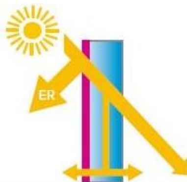
Figure 2.30 Energy reflection effect of reflective coating [29].
