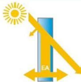
Figure 2.29 Energy absorption effect of tinted glass [33].
