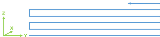
Fig. 2 Path planning for weld. The welding direction alternates with each layer. The first layer is welded in -Y direction. The welding process is stopped at the end of each layer. After a cooling phase of 30 s, the welding torch is moved by the layer height in the Z direction. The second layer is welded in the +Y direction opposite of the first layer. The welding direction changes with every layer
