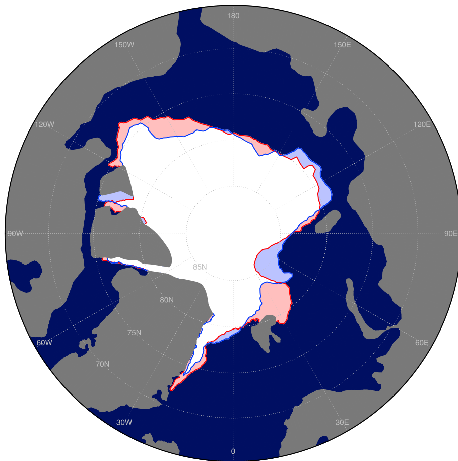
Figure 1. The sea ice edges (15% ice concentration contours) for two members of an AWI-CM idealized forecast ensemble on 15 September (initialized on 1 July of the same arbitrary year). Interpreting the blue contour as forecast and the red contour as truth (observations), the IIEE is the sum of all light blue (ice extent overestimated; O ) and light red (ice extent underestimated; U ) areas, compare equations (1)–(3). The depicted land-sea distribution corresponds to the AWI-CM ocean grid.
