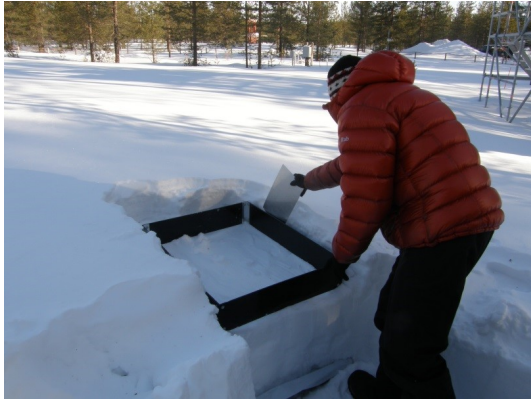
Figure 1. Snow sample was taken from snowpack with a plastic frame, a metal plate and a saw, and a metal bottom plate surrounded by a plastic sheet.
