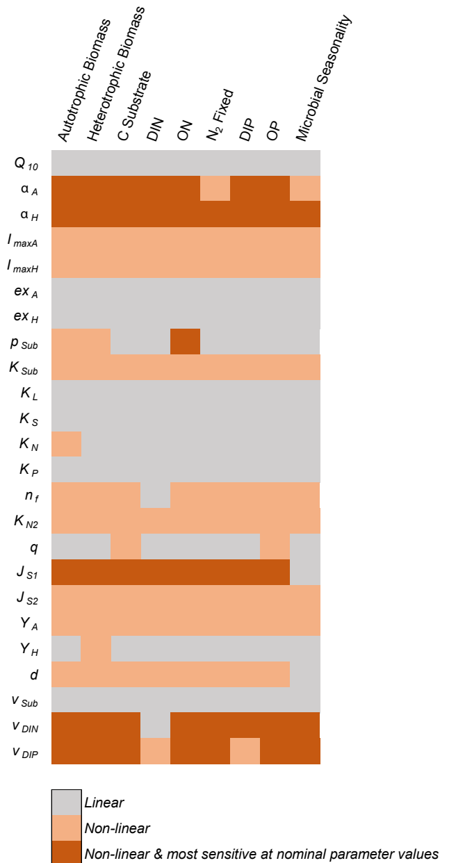
Figure 9. Heat map showing parameter linearity and non-linearity over a range of model outputs. The model is forced with meteorological data from the Damma Glacier (Fig. 4) over 75 years.
