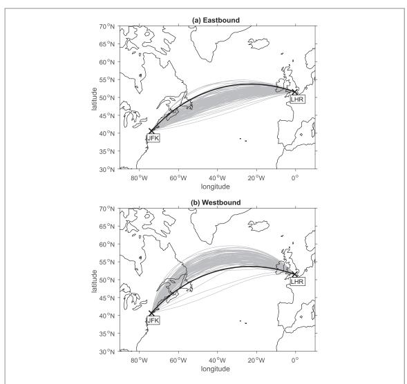
**Figure 3.** Minimum-time routes between JFK and LHR. The 90 grey lines in each panel indicate the daily (a) eastbound and (b) westbound minimum-time routes at the 200 hPa level. The routes are calculated using a pre-industrial control simulation from the GFDL CM2.1 climate model over one winter (from 1 December to 28 February). The black lines indicate the great circle route.
