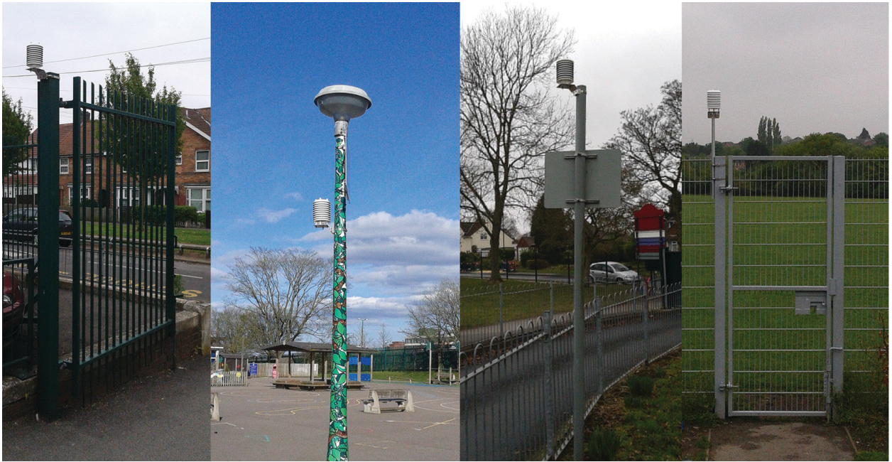
FIG. 4. Photographs of ASMs in typical installations including a gate, a lamppost, a school sign, and an extension pole attached to a fence.
