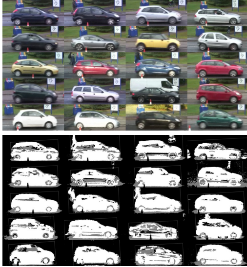
Figure 2: Examples of the normalised RGB and foreground mask composing the vehicle dataset.
