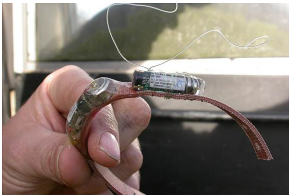
Figure 9 The positioning of the TDR on the collar. The image shows how the TDR is fitted to the collar using fishing line. Prior to deployment it is also covered with protective plastic tubing; it is important that the pressure sensor is recessed within the tubing to protect it from damage. Photo: Andrew L. Harrington.
