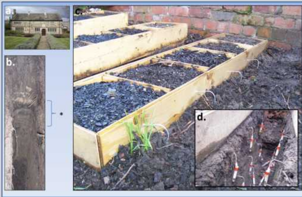
838 Figure 9. Urban soil study site showing a.) view of the garden where experimental trenches were 839 located, b.) excavated soil profile revealing now buried deposits of heavy metal rich soot at the 840 surface of the soil circa. industrial era (marked *), c.) surface amendment matrices and d.) pore 841 water samplers in place at 25, 50 and 75 cm depth.
