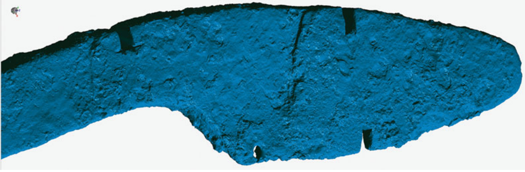
Figure 10. Laser-scanned image showing stress-distortion to the blade and shoulder section of the coulter.
