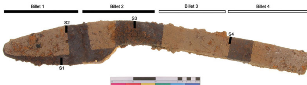
Figure 7. Locations of metallographic sections and the iron billets used in the construction of the coultter; billets 1–2, marked in solid boxes, are based upon visible weld-lines, whereas billets 3–4 (open boxes) are inferred from metallographic analysis.
