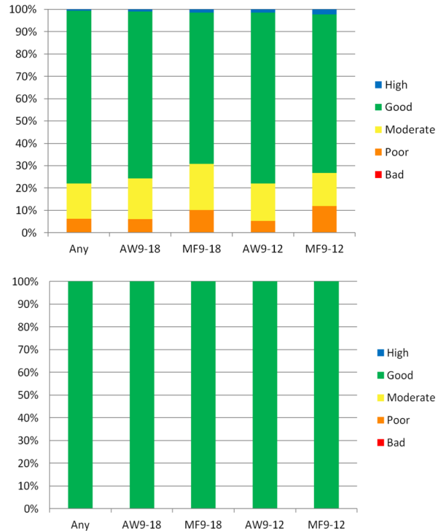
Figure 7. The probability that sampling TRP on the River Kennet for 1 year would put the river into a given WFD class, (a) monthly sampling, and (b) weekly sampling. Strategy labels: Any – at any time; AW9-18, all week, working hours (09:00 to 17:59); MF9-18, Monday to Friday, working hours; AW9-12, all week, 09:00 to 11:59; and MF9-12, Monday to Friday, 09:00 to 11:59.
