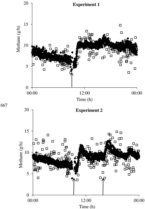
**Fig 2.** Comparison of methane emission rate (g/h; minute average) measured using GreenFeed (GF; open square symbol) and respiration chambers (RC; closed diamond symbol) for all dairy heifers in experiments 1 (n = 8) and 2 (n = 16). There were 56 d GF and 32 d RC measurements for experiment 1, and 112 d GF and 64 d RC for experiment 2. Arrows indicate time of feeding.
