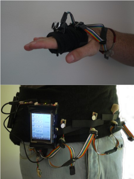
Fig 4. TESSA in glove configuration (top) and belt configuration (bottom)
