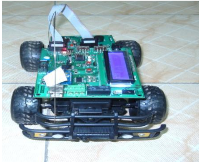
Fig. 2. The proposed mobile sink – a classical vehicular robot design.
