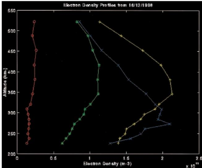
**Fig. 3.** Altitude profiles of electron concentration,  $N_e$ , for four one-minute integrations of the ESR data. *Blue* ( $\times$ ): 06:16–17 UT, when the ESR was at sub-auroral latitudes. *Yellow* ( $+$ ): 06:52–53, when the ESR was within the cusp/cleft transient *f*. *Green* ( $*$ ): 06:56–57 when the ESR was between cusp/cleft transients *f* and *g* (the time marked with the *arrow* in Fig. 2). *Red* ( $o$ ): 07:15–16 UT when the ESR was within the polar cap
