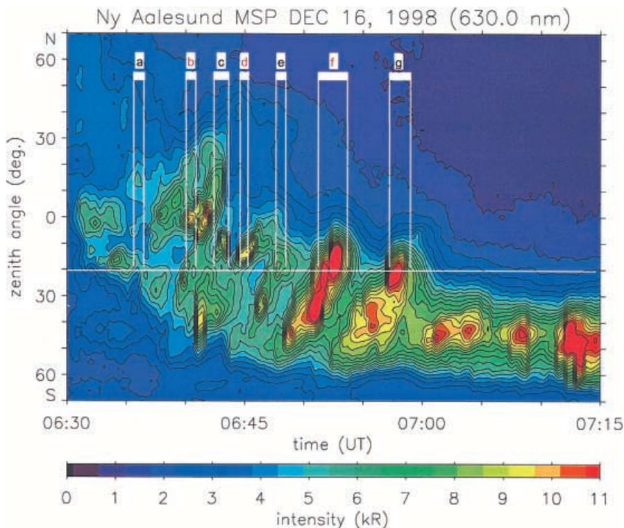
**Fig. 1.** Integral line-of-sight intensity of 630 nm emissions, as seen by the 630 nm meridian-scanning photometer at Ny Ålesund, colour-coded as a function of zenith angle and time. The horizontal line shows the zenith angle of the ESR radar beam for an assumed emission altitude of 300 km. The passages of poleward-moving events through this approximate location of the ESR beam are marked as events *a–g*
