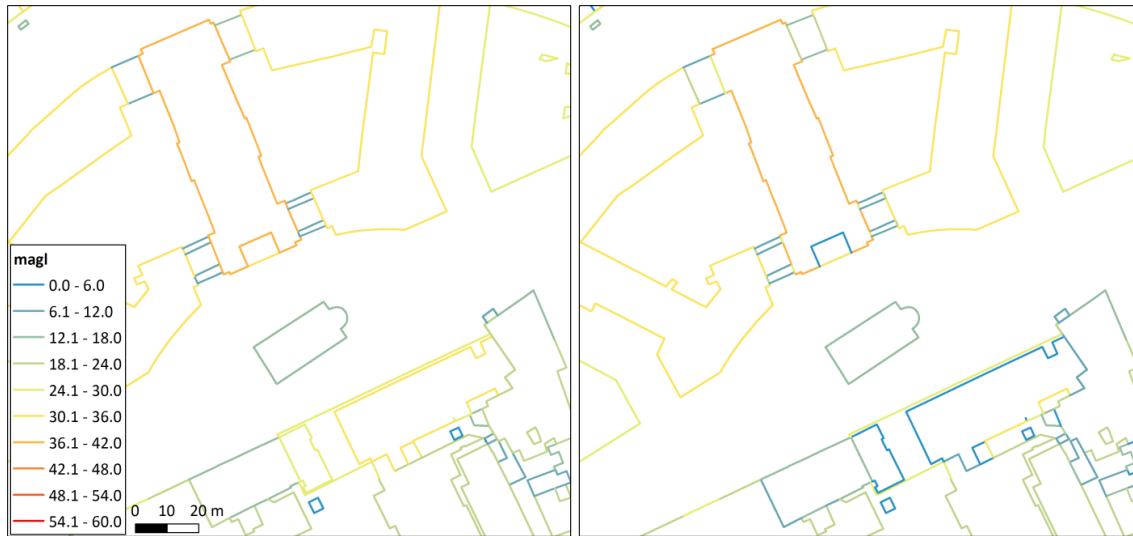
Figure A1: Wall heights represented as left ; height above ground level and right ; height difference between ground or adjacent building.
