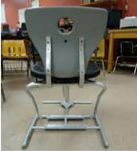
Figure 17. Fabricated seat and back support mounts.
