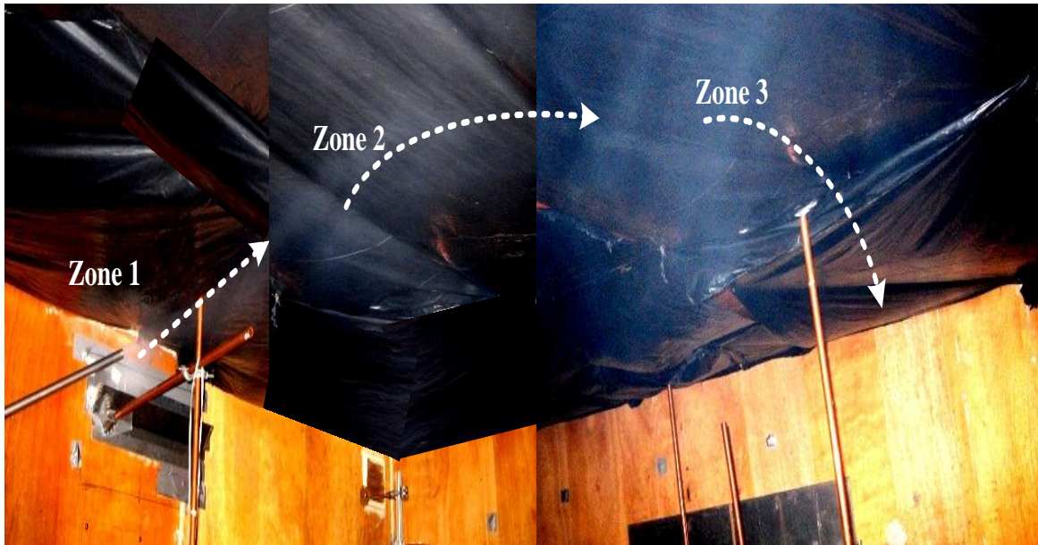
Figure 7 Smoke visualisation test showing the flow from the inlet supply.
