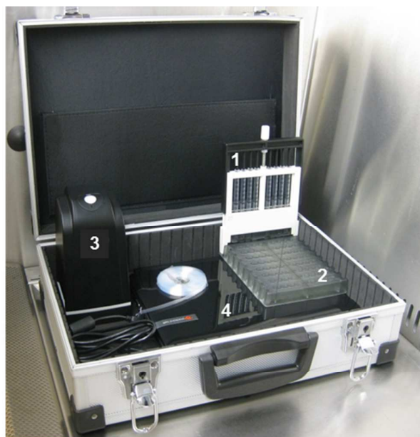
Figure 1. Main components of "Lab-in-a-briefcase" for PSA screening.
