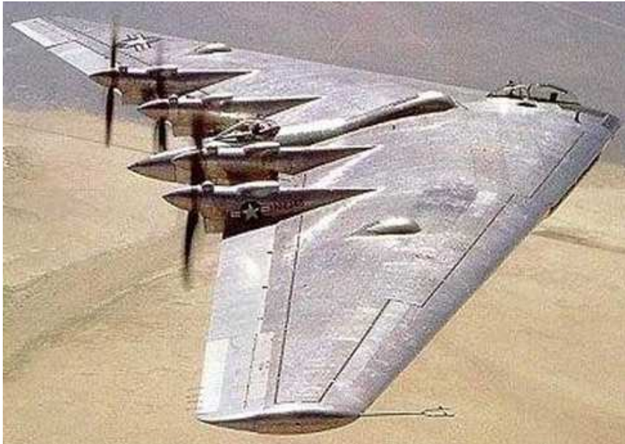
Figure 2.6: Northrop XB - 35 Piston - engined Long - range Bomber (Source: Virtual Aircraft Museum).
