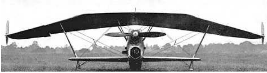
Figure 2.2: Westland-Hill Pterodactyl V Aircraft with Fully Moving Wingtips[15].
