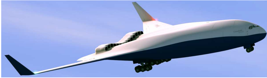
Figure 2.21: Cranfield BWB Design showing the BLI Distributed Propulsion System. (Source:Cranfield Aircraft Design Group).
